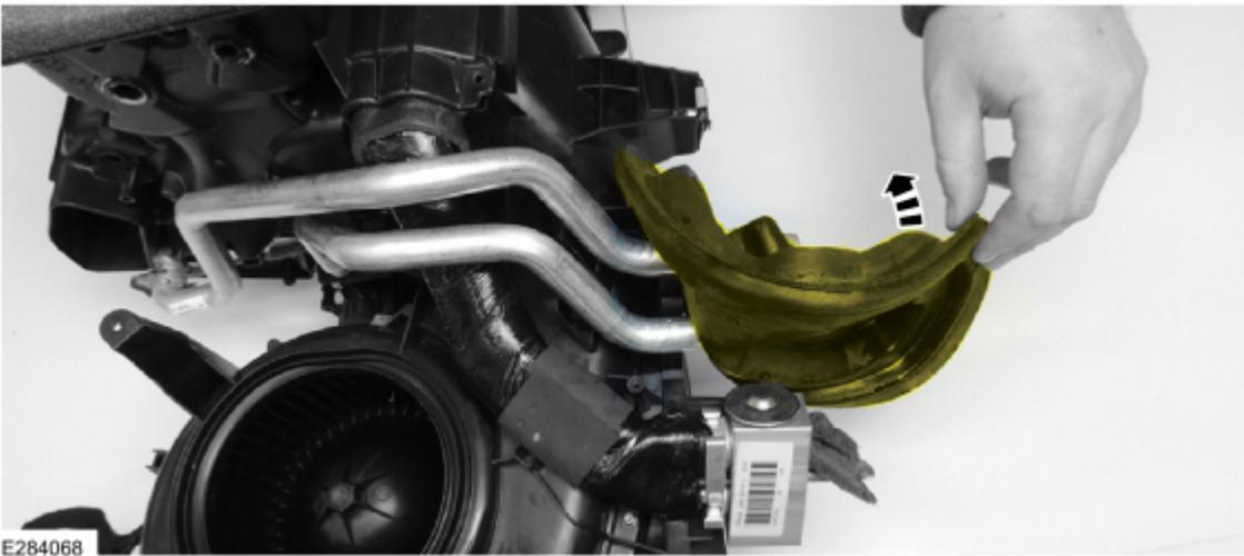
**14.** Remove the plenum chamber and heater core as an assembly from the climate control core housing. (Figure 13)
