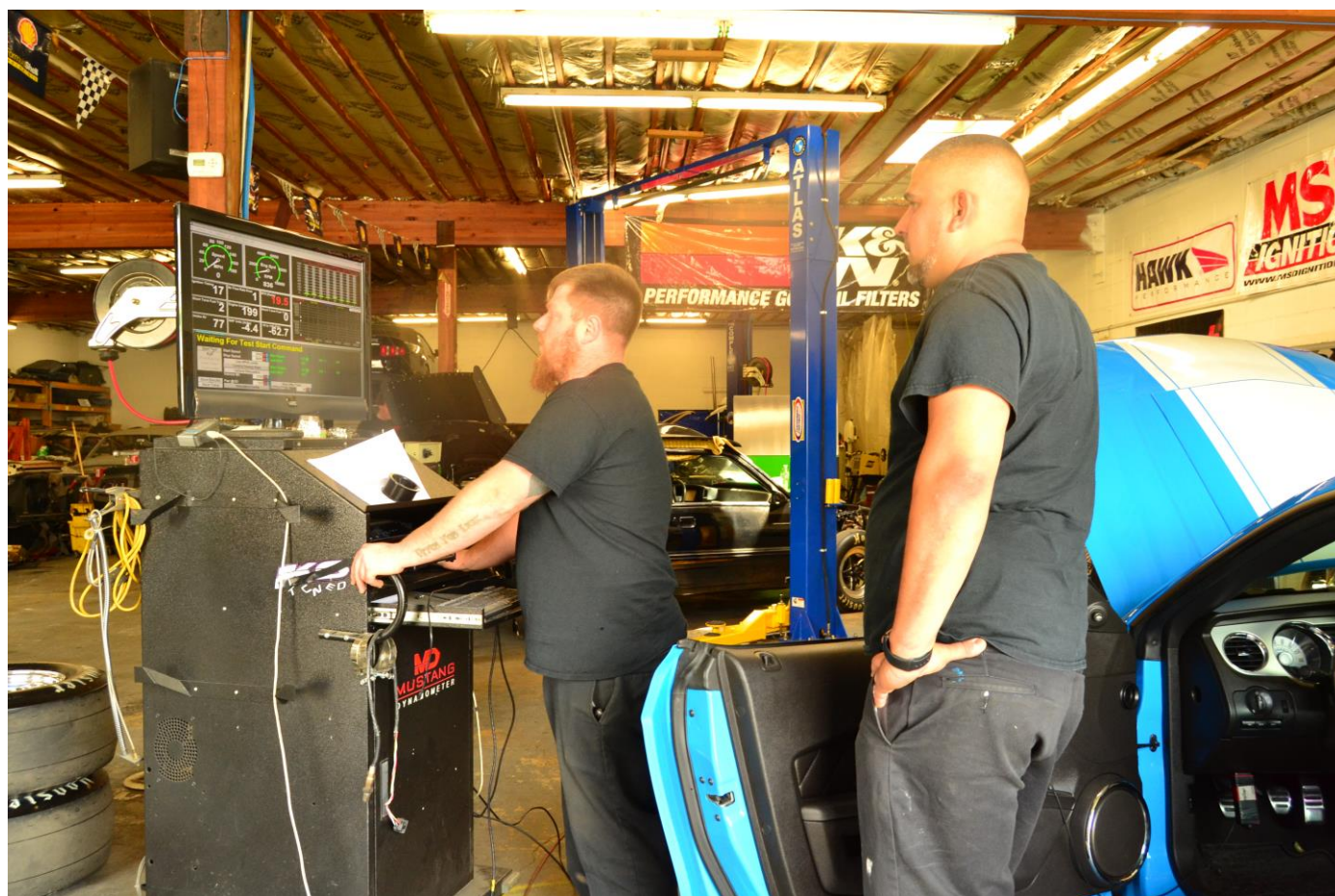
Figure 4. Data collection from a chassis dynamometer at The Mustang Shop (TMS) in Kent, WA. Light blue test vehicle can be in the bottom right of the photo.
