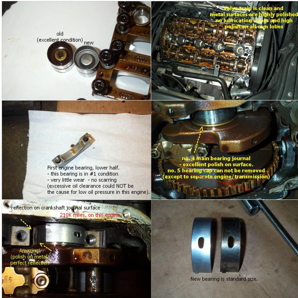
Figure 3. Selected pictures from the report provided by a mechanic. With 210K miles on the engine, MHS powder was added at 208K miles. Results were achieved in about 40 motor hours. He extracted hydraulic lifters and main journal bearings for further analysis. Our mechanic described formed film as “polish” and could not hide his admiration of the mirror smooth surfaces.
