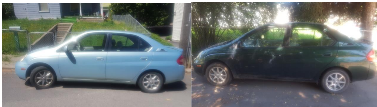
Figure 7. Two 1 st generation Toyota Prius test vehicles: blue baseline vehicle (left), odometer reading 160k miles, and the green vehicle with one application to the engine oil compartment of TriboTEX nanomaterial engine coating (right), odometer reading 203k miles.
