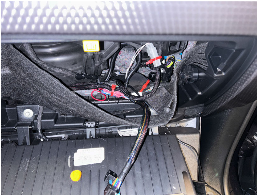
View of connectors behind dash, behind glovebox with felt removed.
