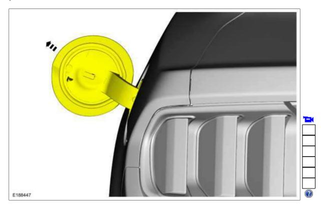
2. Using a screwdriver, pry the retaining tab back and slide the fuel filler door from the fuel filler door hinge.
