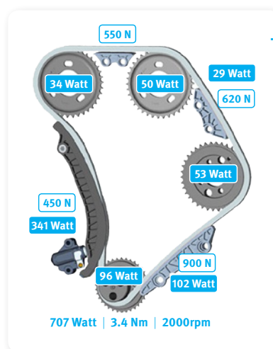
Figure 1. A timing chain layout with parasitic loss contributions due to sliding friction and chain articulation.
