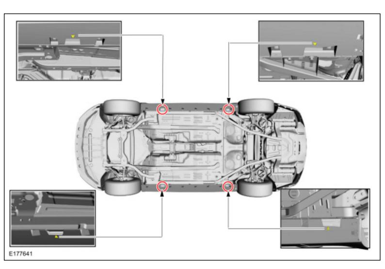
Only the specified jacking points may be used for jacking and supporting the vehicle.
