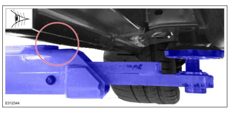
NOTICE: Use spacer blocks to increase the clearance between rocker moulding and the hoist arm.
