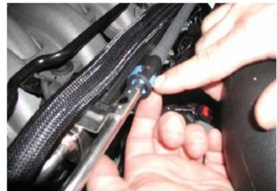
Disconnect Fuel Supply Line
