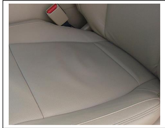
Figure 2 – Misaligned/loose seat trim covers must be corrected through adjustment. Refer to WSM Section 501-10. Stretching/looseness of the seat cushion cover center panel is a characteristic of leather seats and may not improve with adjustment
