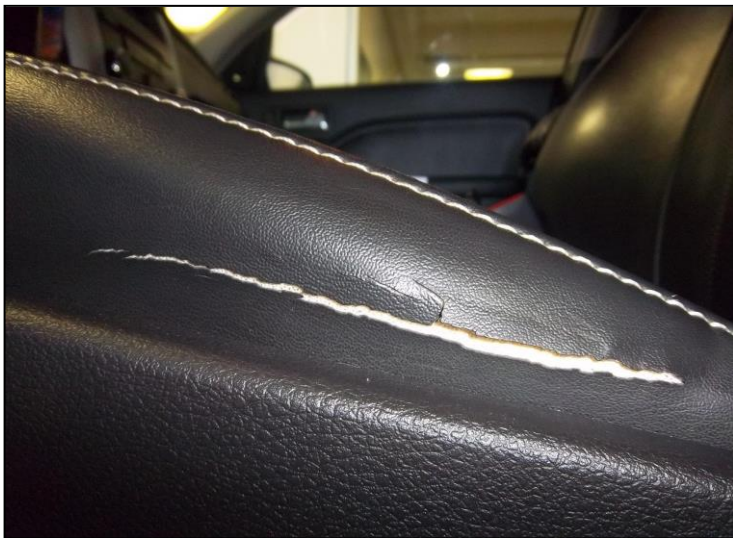
Figure 17 – Cracking on side bolster (jagged lines) not caused by cuts/snags
