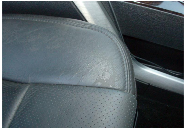
Figure 10 – Failed repair attempt such as vinyl dye/painting, evidenced by smooth/shiny surface and lack of the natural leather grain. Overspray on thread or other panels is an indication of vinyl dye/painting
