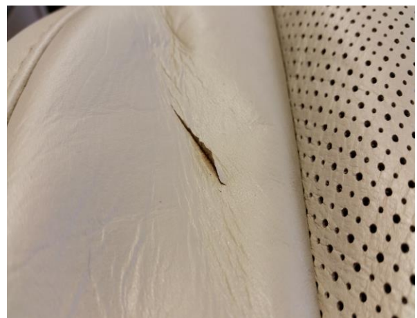
Figure 6 – Cut in leather (mistaken as leather top coat peeling) leather russet still attached to underside of top coat
