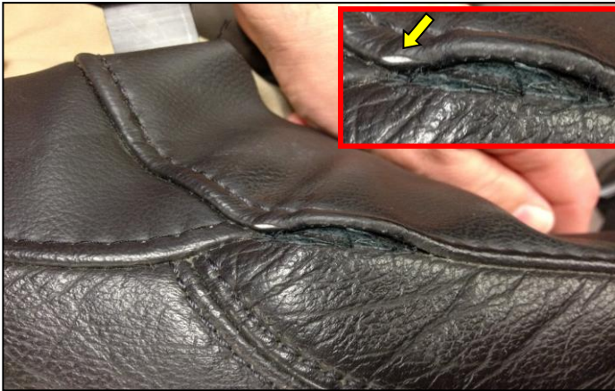
Figure 3 – Split seam with evidence of cuts, scratches, snags, puncture or stain marks to surrounding material or thread.
