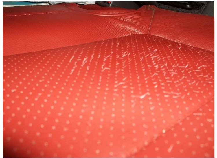
Figure 22 – Bearding is the result of the foam backing rubbing the backside of the cover, causing fibers from the backing to come through the perforations in the leather
