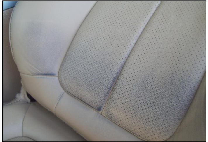
Figure 12 – Dye (colors may vary) transfer from clothing resulting in discoloration
