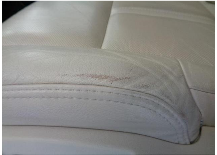
Figure 16 – Ingress/Egress Wear Top/Color coat is worn (smoothly not scratched) off from entering/exiting the vehicle. Leather subsurface is visible. Tip: Leather russet will darken when wiped with a damp cloth
