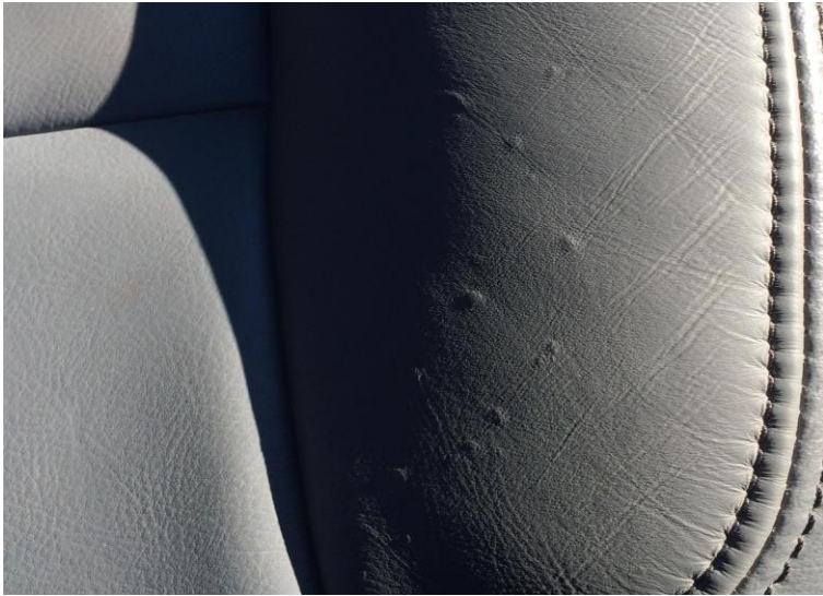
Figure 21 – Bumps/blisters on the surface
