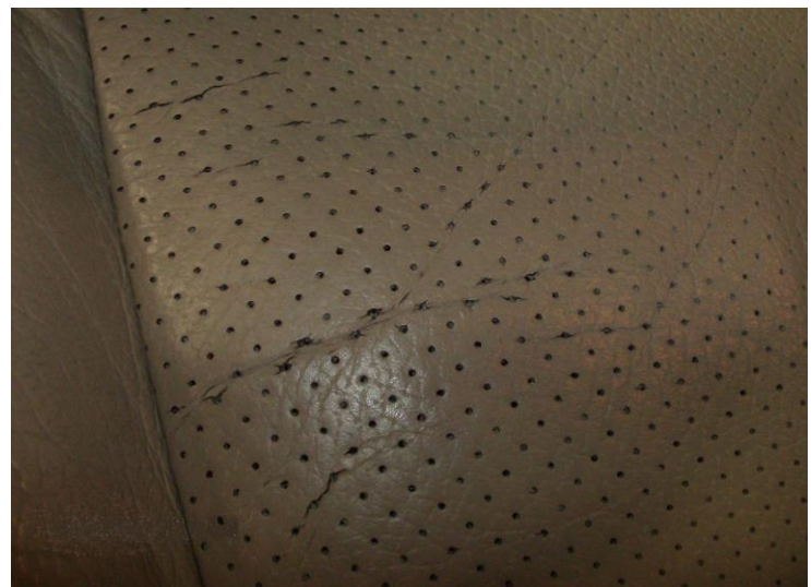
Figure 18 – Cracking between perforations not caused by cuts/snags/chemical damage
