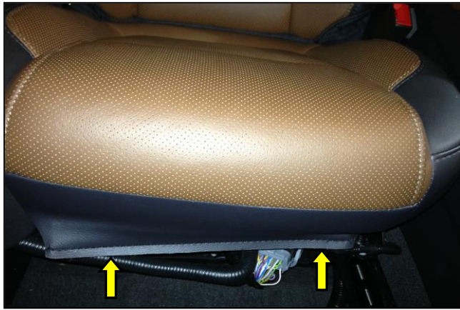
Figure 1 – Loose seat trim cover typically caused from loose/detached retention J-clips. Loose J-clips can be repaired/re-attached per Warranty and Policy Manual. J-clip loose from material can be re-sewn
