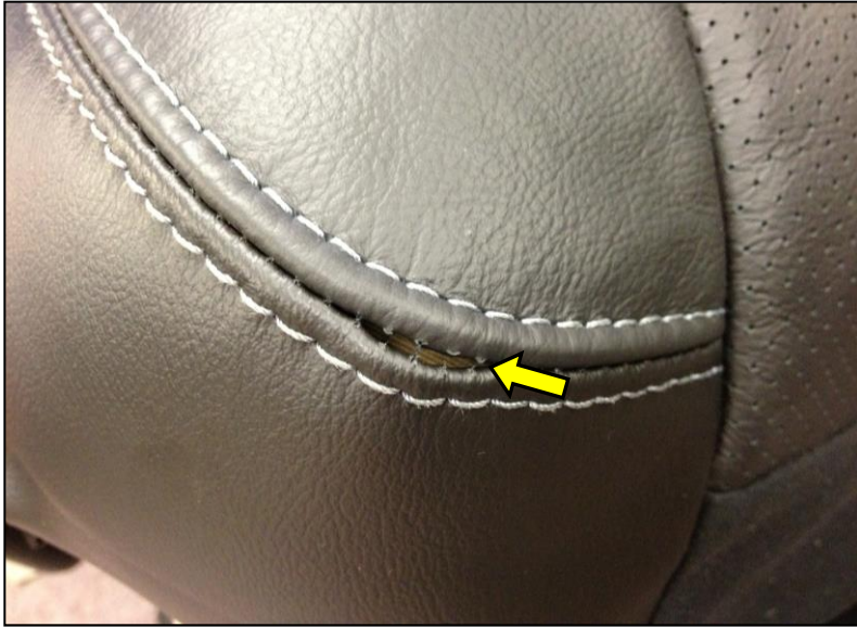
Figure 19 – Split seam with no evidence of staining/cuts/scratches/damage to threads and surrounding area
