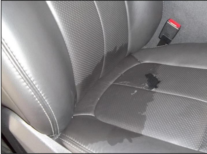
Figure 7 – Chemical damage resulting in discoloration typically across multiple panels and or a peeling surface
