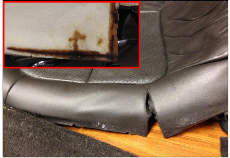
Figure 8 –Seams split caused by chemicals which break down stitching
