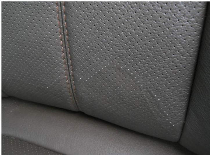
Figure 9 - Liquid Damage that spans across multiple leather panels that may appear to be a natural scar. Once a liquid is allowed to soak in the leather and then left to dry, a raised edge may appear that feels rough to the touch
