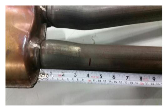
6. Slide the X-pipe into <u>RH</u> catalytic converter and <u>LH</u> muffler inlet pipe clamps. Making sure to center the clamps between the two pipes. Snug both clamps to hold X-pipe in place.
