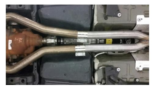
9. Align system in rear facial and torque factory clamps to 35 lb.ft (48 Nm) and the supplied clamps to 40 lb ft (50Nm)
