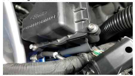
14. Push the end of the short hose to the PCV valve on the valve cover. Attach the long braided hose with the 45 deg. fittings to the outlet port on the separator and attach the other end to the intake manifold port. Check that all hose ends are locked and installed properly.
