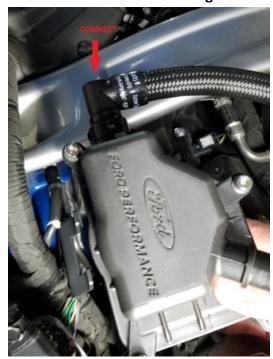
13. Tuck the fitting under the strut tower brace (if present) and slide the oil separator onto the mounting brackets tabs.
