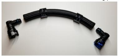
4. Slip 2 Gates heat shrink clamps over the long braided hose. Insert the 45 degree fittings on each end as shown. 45 DEGREE FITTINGS MUST GO ON THE LONG HOSE.
