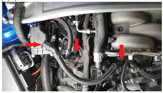
15. Installation of the oil separator is now complete.
