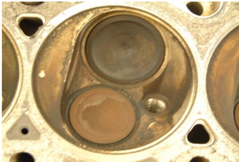
Figure 25. Intake and exhaust valves from Clear- and MMT-vehicles.
