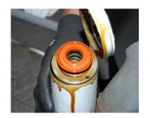
Step 3 – Cut element from filter
