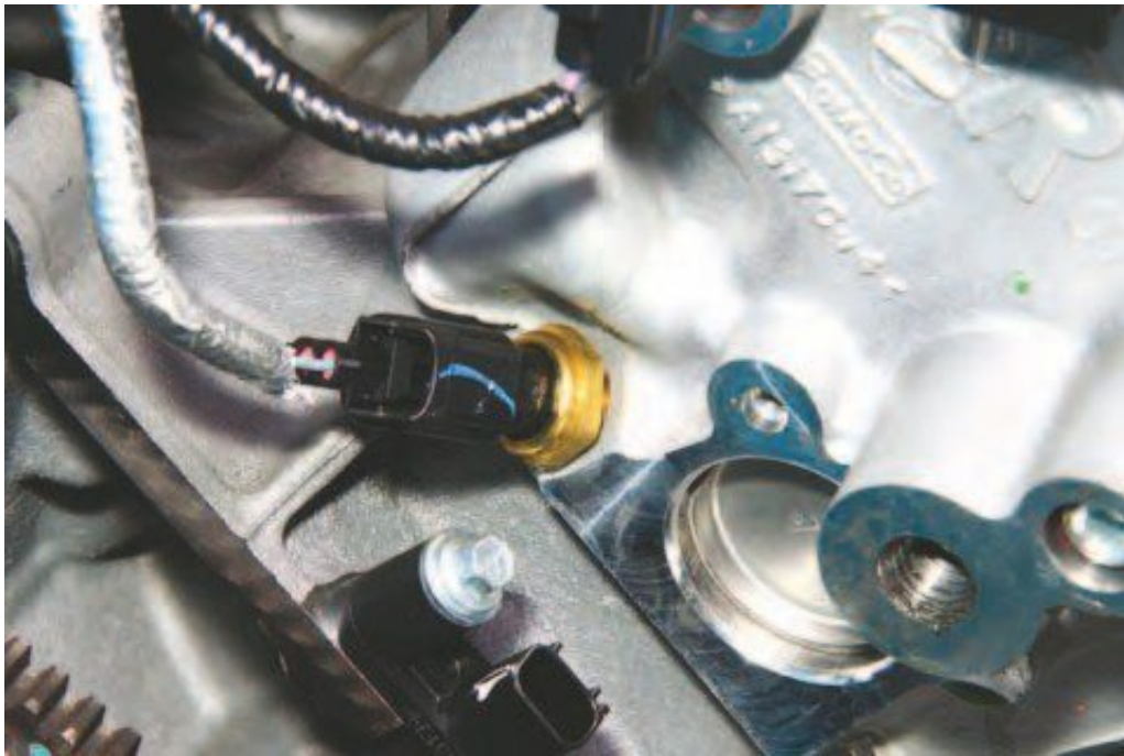
This is the cylinder-head temperature sensor, which contributes to the electronic engine control picture and temperature gauge.
