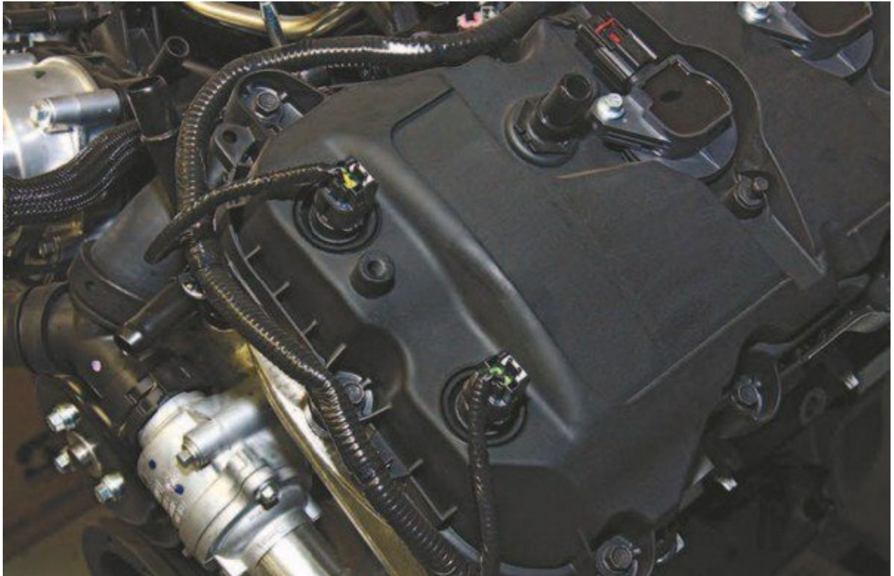
These are the Ti-VCT solenoid connections for variable cam timing. These solenoids modulate the VCT valves to advance valve timing. Each cylinder bank has two of these solenoid valves: one for intake and one for exhaust cam indexing. This is the left-hand (driver) bank.
