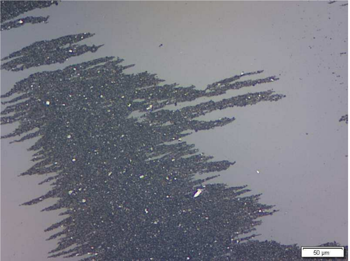
CORROSIVE WEAR 500X
