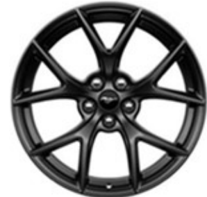
19" X 9.5" Magnetic-painted Aluminum Included in EcoBoost® Handling Package (60H)
