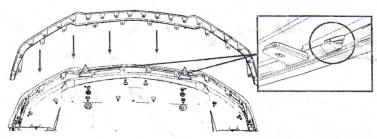
Install (8) W716492-S450B Black M6 Bolt from Step 2 securing the Splitter, Front Fascia, and Lower Strikes (four outboard secures) to the Belly Pan. Torque to 8 Nm.
