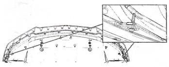
6. Install (2) W520802-S307 Black M6 J-Clip to the outboard wheel liner flap, one on each wheel liner.
