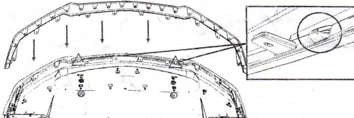
4. Install (8) W716492-S450B Black M6 Bolt from Step 2 securing the Splitter, Front Fascia, and Lower Strikes (four outboard secures) to the Belly Pan. Torque to 8 Nm.
