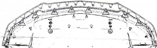
5. Install (2) W716492-S450B Black M6 Bolt securing Lower Strike and Front Fascia to Splitter. Torque to 8 Nm.
