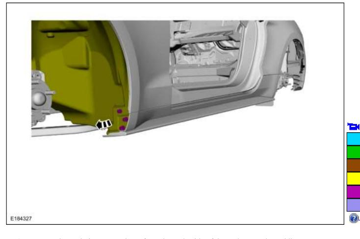
2. Remove the pushpin type retainers from the underside of the rocker panel moulding.
