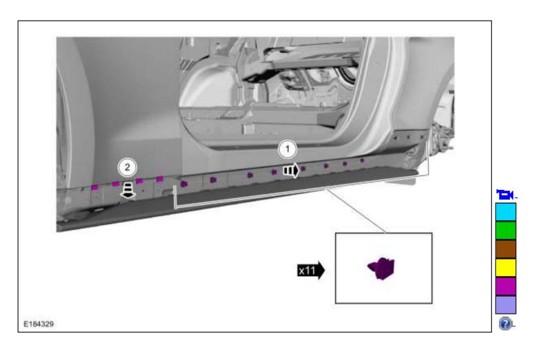
4. Remove the rocker panel moulding.
