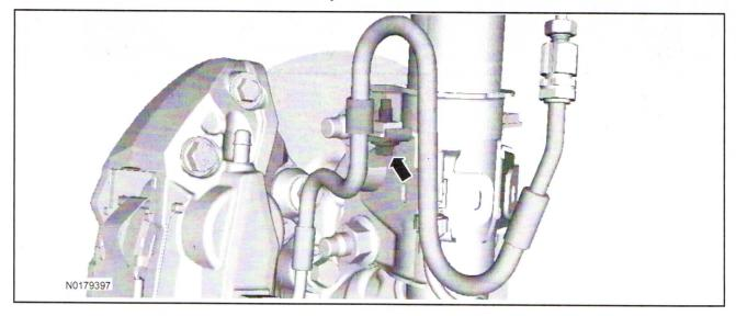
6. If equipped with dynamic suspension, disconnect the dynamic suspension strut wire harness connector.
