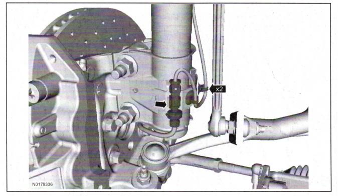
20. If equipped with dynamic suspension, connect the dynamic suspension strut wire harness connector.
