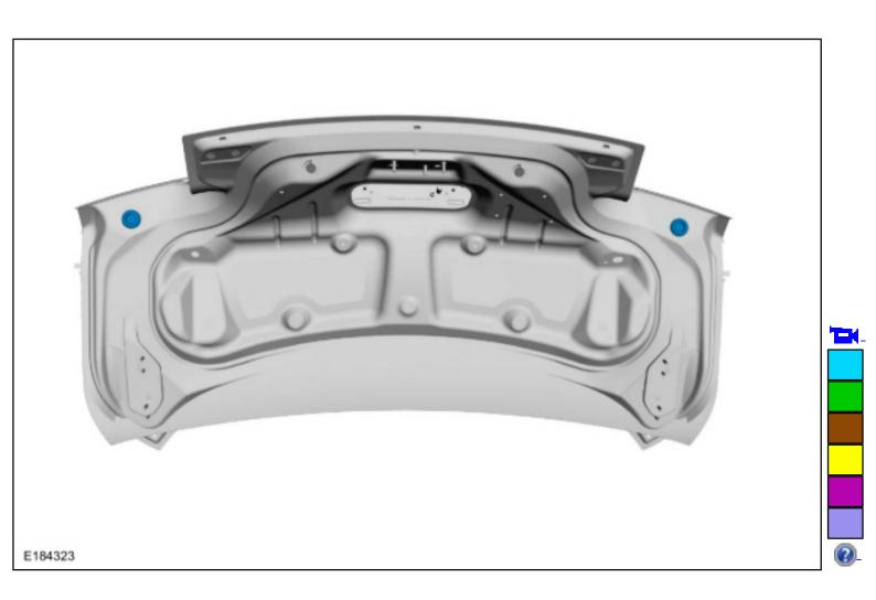
3. Remove the nuts. *Torque*: 48 lb.in (5.4 Nm)
