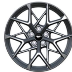
10.5" (F) 19" X 11" (R) Tarnished Dark-painted Aluminum Available on the Handling Package (60K) "Late Availability"
