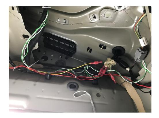
7. I ran the GND wires to the grounding point on left center left center rear of trunk as shown in the diagram above, already used by several other devices.
