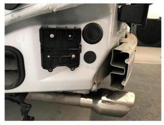
4. Mount SODL/R and connect pigtails. I couldn't find any used connectors for Mustangs, so I ordered a pair of new ones from rockauto.com for less than \$17 each. I removed unused pins and labeled the wires using the wiring diagram below. Note that connectors also come with pin numbers for reference.
