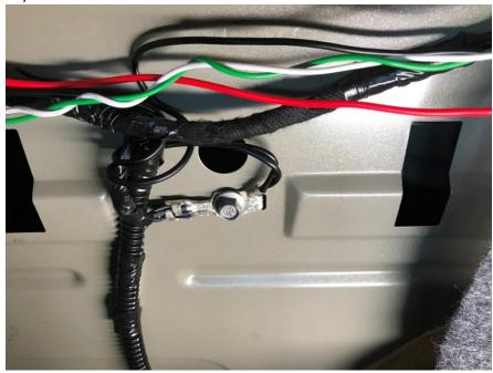
8. I have a coupe, so the Body Control Module B (BCMB) is on the right side of the trunk. The black harness contains pin #11 (GRY) for MS CAN+ and #23 (VIO) for MS CAN-. Unlike other pins, two thinner wires share one pin each as shown in the wiring diagram. It doesn't matter which wire you tap into as long as the polarity matches.
