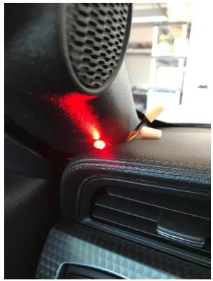
7. For the CTA test, I placed the car in the driveway with the parking brake set while in reverse. A friend drove down the street from the left to the right side. Left-side warning came on first with sound and switched to the right-side warning as he passed the car and continued down to the right side until he was out of the range.
