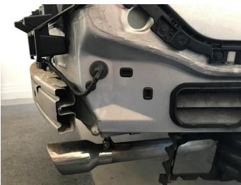
3. Install mounting brackets. Existing mounting hole covers didn't have provisions to attach the brackets, so I flipped the covers around and used nuts and bolts to secure the brackets with added double-sided tape on corners without holes.
