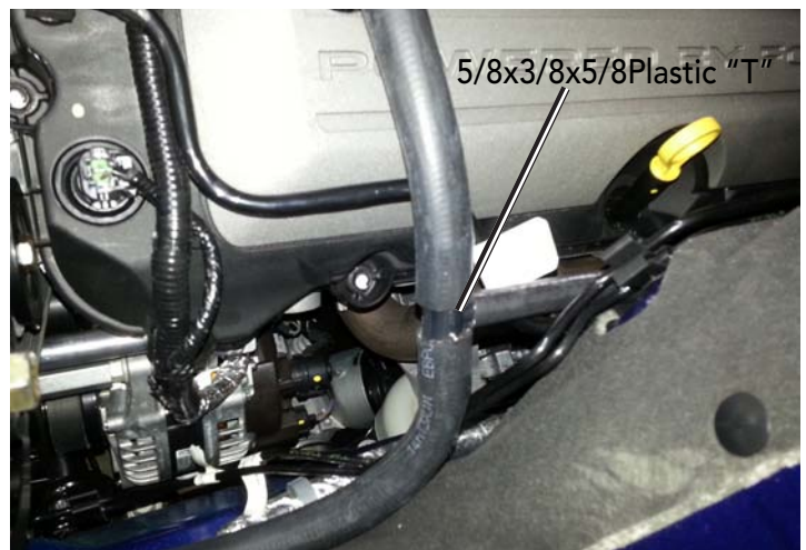
Plastic "T" In Driver's Side PCV Hose
