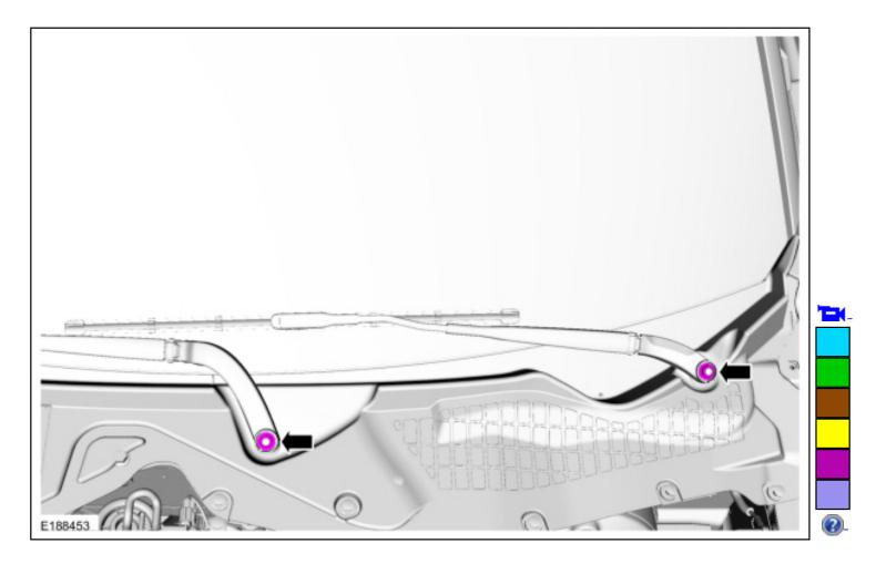
3. Remove the windshield wiper pivot arms. Use the General Equipment: Two Leg Puller
