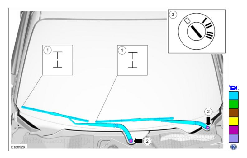
3. Install the windshield wiper pivot arm nut covers.
