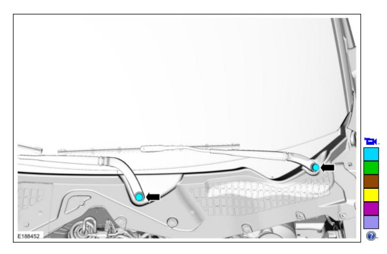
Remove the windshield wiper pivot arm nuts. *Torque*: 26 lb.ft (35 Nm)
